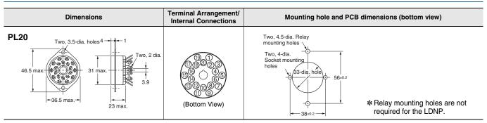
Note: When mounting, pay due attention to the direction of the key groove of applicable Relays.
