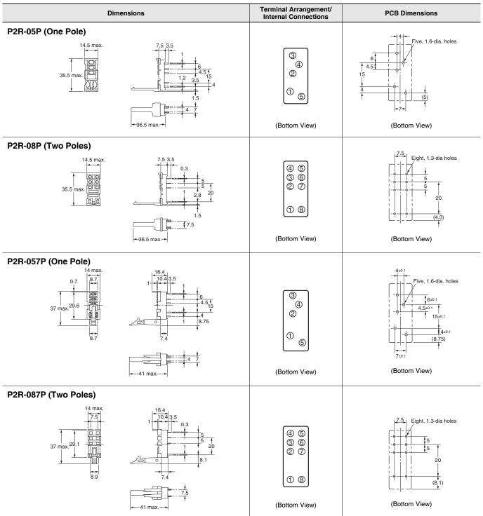
Note: If an I/O SSR or Indicator Module is used, the polarity of terminal 1 is negative.
