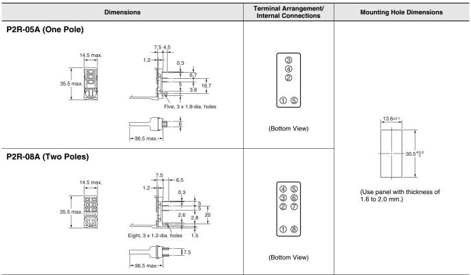
Note: If an I/O SSR or Indicator Module is used, the polarity of terminal 1 is negative.
